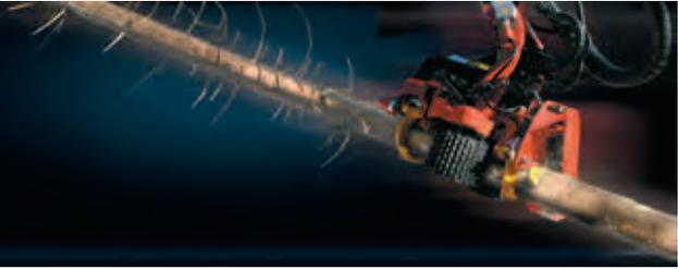
SPd5Bucking is a complete measuring and operating system for controlling the felling process in a harvester head. SPd5Bucking is our most advanced system, with support for bucking to value. The system is also entirely integrated with the dasa5 operation and communication system.
